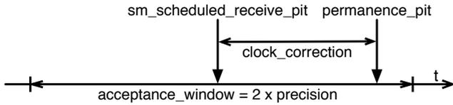
**Figure 3: Clock correction in synchronisation master and client.**
