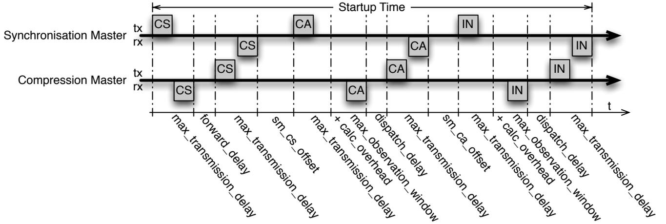
Figure 6: Estimation of startup time (time to sync).
