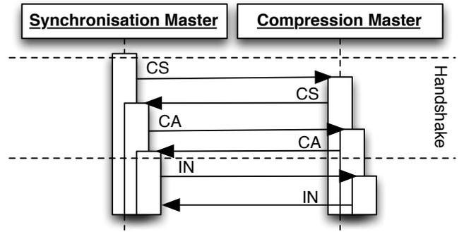
**Figure 2: Startup sequence: After initial synchronisation has been done by the handshake protocol, the synchronisation master sends the first integration frame to the compression master. The compression master generates a new integration frame in response and sends it back to the synchronisation master.**
