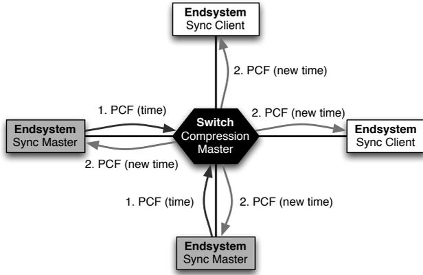
**Figure 1: Two step synchronisation approach: Protocol Control Frames of type IN are sent by the synchronisation masters to the compression master, the compressed time is then calculated and propagated to all of the systems participants.**
