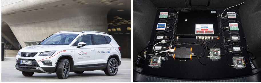
Fig. 8: SecVI prototype with security-enhanced network installed in the trunk.
